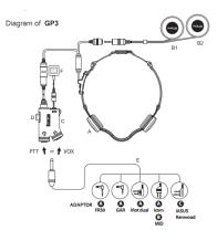
Transponder Α B1, B2 Helmet speakers DIN plug D PTT/VOX splitter Ε Adaptor wire PTT switch
