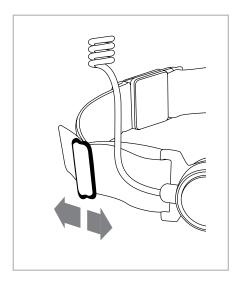
III. Adjust the neck strap for tightness by using the adjusters (E). The throat mic needs to be just snug but not tight around your neck.
