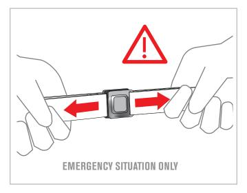
In the event of an emergency where removal of the NT3-R is required, pulling the neck strap apart in opposite directions will quickly disengage the clasp.
