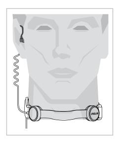
II. Place the throat mic around your neck and reapply the clasp so that it makes contact all around.
