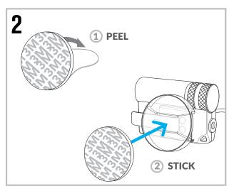
Peel away the backing paper on the 3M Adhesive (H) and position in on the Quick Release Mount (G)
