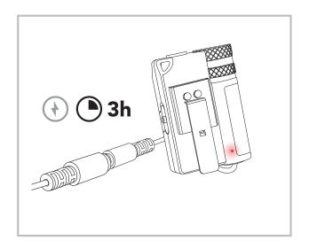
When charging, the Charging Indicator LED (7) is lit red and will turn off when charging completed. A full charge can be completed in about 3 hours when charged using a computer's USB port (0.5A output). Each charge allows for usage of up to 20 hours, depending on the output volume level and ambient temperature.
