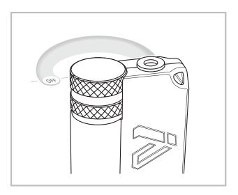
The EAR3H is equipped with the IASUS signature CNC-machined and knurled aluminum volume knob for an enhanced grip, even when operating with gloves.
