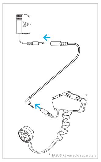
Connect the Audio Source into the Input jack (3) of the EAR3H Amp.
