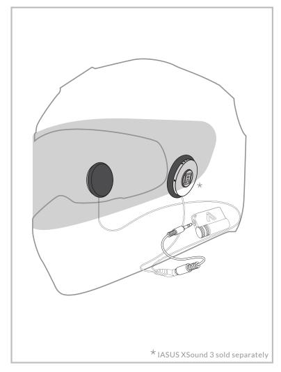
If needed, use the included short extension cable. For a tidy installation, cables can be tucked behind the helmet padding.
