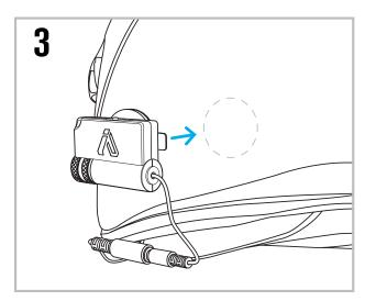
Peel the second backing paper on the 3M Adhesive. Position on your helmet and press firmly.
