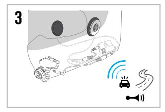
Put on the helmet and adjust EAR3H volume for ambient sounds by slowly turning the volume knob.
