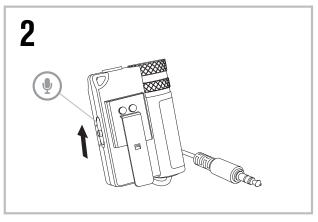
On the side of the EAR3H, slide the TRANSPARENCY MODE switch to the ON position.
