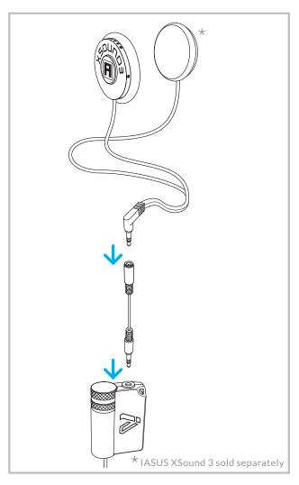
Connect helmet speakers, or earphones directly into the Output jack (4) of the EAR3H Amp.
