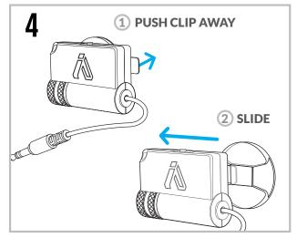
To remove EAR3H from the mount, simply push the clip away from the amp and slide the unit until it is fully released.
