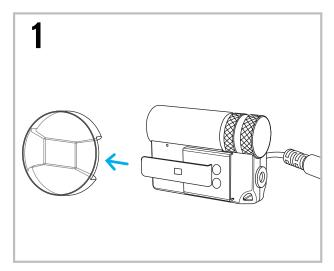
Clean the mounting surface of your helmet. Secure the EAR3H onto the Quick Release Mount (G).
