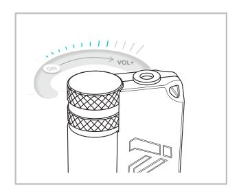
Power on the amp and continue turning clockwise to your desired volume level.
