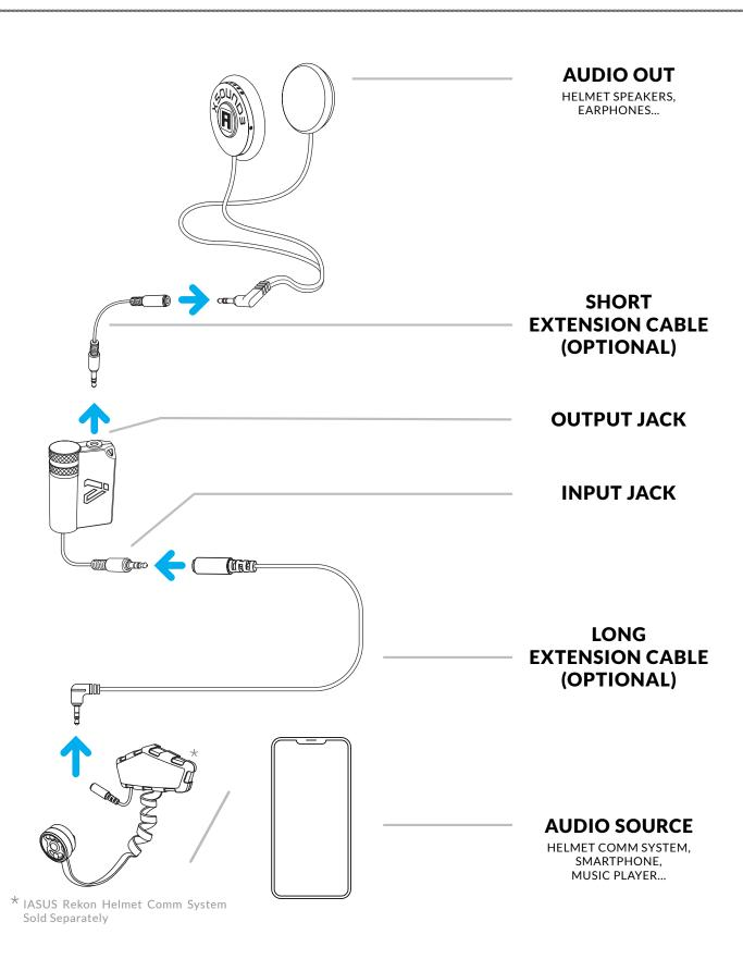
**Note:** While the EAR3H Output Jack supports headsets and earbuds with an inline mic, any mic input will not pass through the EAR3 and into the audio source. A smartphone will not receive any input from that mic.
