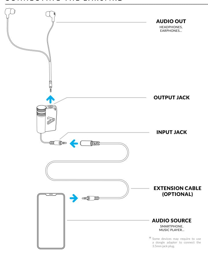
**Note:** While the EAR3MK2 Output Jack supports headsets and earbuds with an inline mic, any mic input will not pass through the Mobile Amp and into the audio source. A smartphone will not receive any input from that mic.
