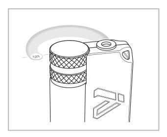
The EAR3MK2 is equipped with the IASUS signature CNC-machined and knurled aluminum volume knob for an enhanced grip, even when operating with gloves.
