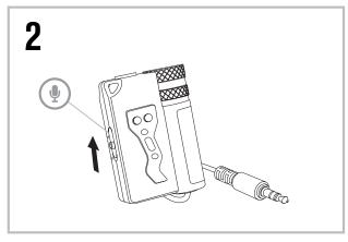
On the side of the EAR3MK2, slide the TRANSPARENCY MODE switch to the ON position.
