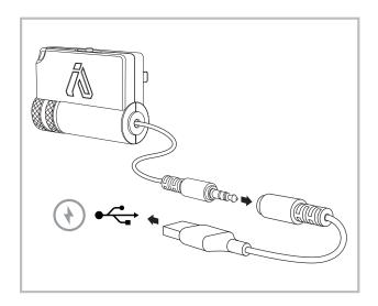
The EAR3MK2 is powered by an internal, non-removable lithium-ion battery. It is pre-charged, enabling the EAR3MK2 to be ready for use right out of the box.
