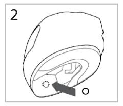
Place the magnetic mount into the chin opening of the helmet. Ensure there is sufficient space for the BMH to adhere to the magnetic mount before pressing firmly for a secure attachment.
