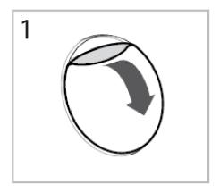
Clean the mounting surface of your helmet. Peel away the backing paper on the BMH Magnetic mount (D).
