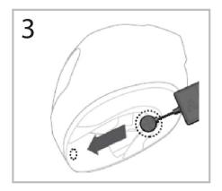
Remove the remaining paper from the velcro mount (C1/C2) that is now attached to the mic. Place the BMH onto the magnetic mount and position the mic inside the helmet directly in front of your mouth for optimal clear audio.
