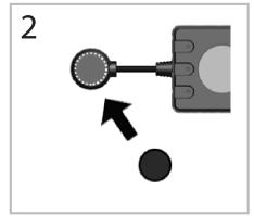
Position the sticky side onto the BMH Microphone (A1). Apply firm pressure to ensure proper adhesion.
