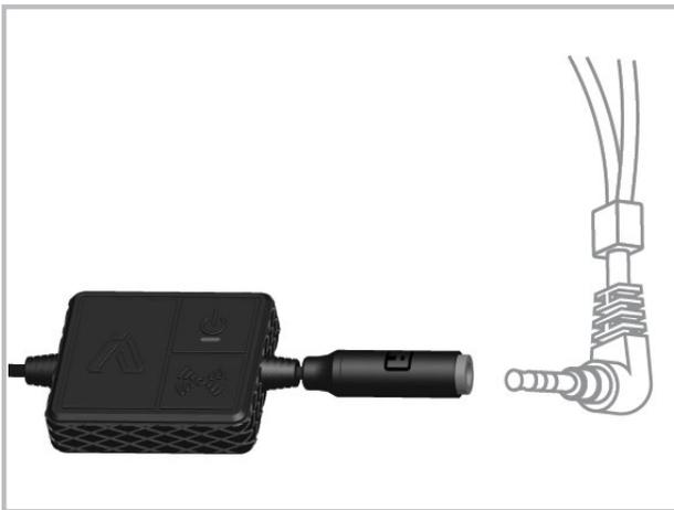
The EAR3H-MK2 Helmet Amplifier is equipped with a 3.5mm audio output connector that is optimized for the following IASUS audio accessories :
