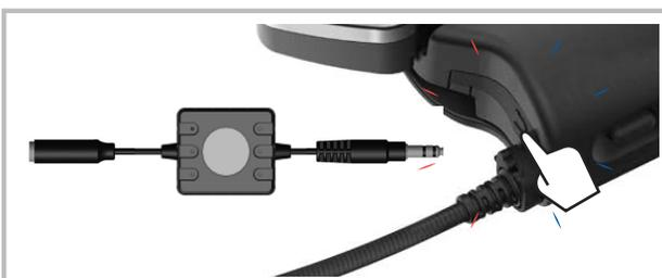
Insert the 3.5mm audio pin into your device's 3.5mm earbud port or jack. Please note, some devices may have an alternative 3.5mm port location, so check for a separate earbud port if needed.
