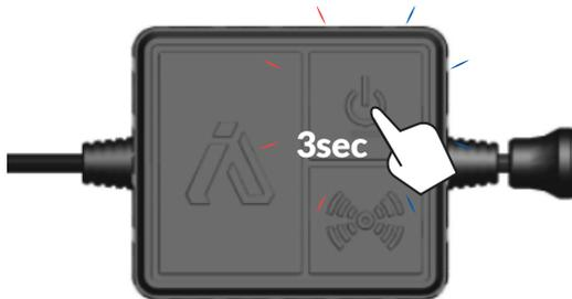
Turn the power on by depressing the power button for 3 sec. Once turned on there will be a continuous green power LED light.
