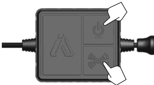
To adjust the volume, simply press the power button for volume up and the wave button for power down. Be careful when using EAR3H, as the volume increase is very significant and to check the input volume level prior to setting up the amp. If input is very loud, the resulting extra amplification could be quite extreme. Best result are to have source volume at about 50% to start and then work your way up. Can adjust both source and amplifier volume for desired level.
